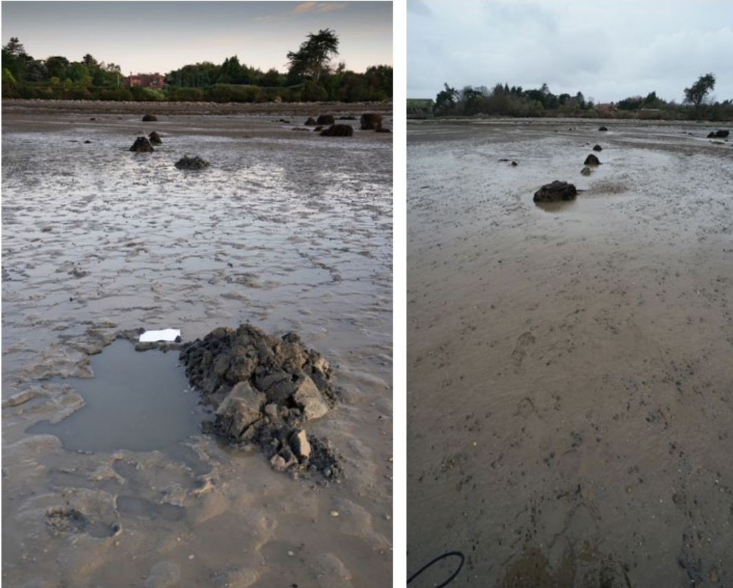
Figure 20 - The control holes on 30/09/2019 (left) and the same area 10/03/2020 (right) 162 days later. The sediment surface has lost its pitted appearance and there are no signs of the control holes
