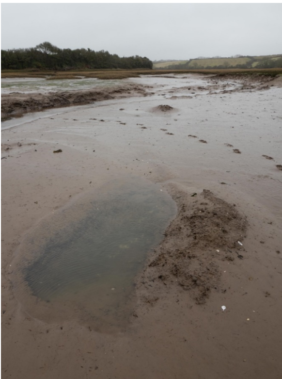
Figure 87 - Control holes still present on 14th March 2020 (107 days) and enlarged by scour
