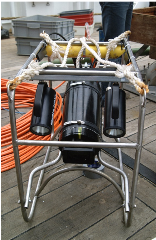
Figure 6. CCW/NRW drop down video sledge ready for deployment.
