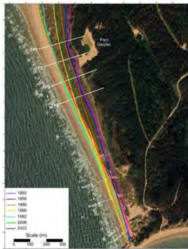
Figure 12. The position of the dune toe estimated from historical aerial photographs. Base satellite imagery flown 04/07/2023 (source: Google Earth). The positions of shore-normal profiles and frontal dune notches referred to later in the report are also shown for reference. Source: Welsh Government Cartographics Dept.
