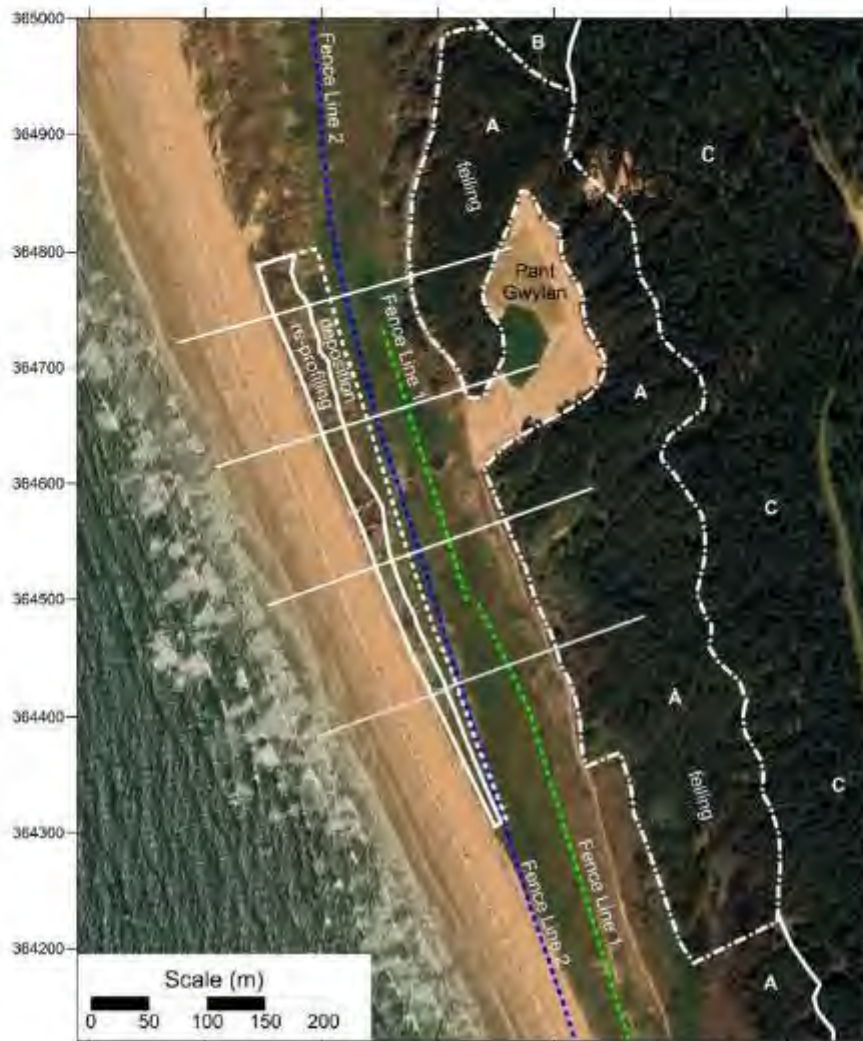
Figure 35. Option G: area of reprofiling (white solid line) and deposition (white dashed line) of sand along the frontal dune, with 10 ha of clear felling behind in the zone identified for “Open Habitat Management” (A) in the 30 year vision Forest Plan (dash-dot-dash white line). Other Forest Management 30 year vision areas are B (successional woodland) and C (native woodland management). Also shown are the lines of fences shown on historical aerial photographs: Fence Line 1 (green dashed line, shown on aerial photographs flown 02/02/1956); Fence Line 2 (blue dashed line, shown on aerial photographs flown 31/05/1960 and 07/06/1966). Base Google Earth satellite imagery flown 04/07/2023.
