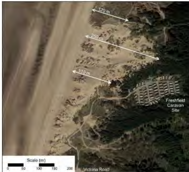
Figure 24. Example of mobile dunes advancing up to 250 m inland into the pine forest north of Victoria Road, Freshfield. Base aerial imagery dated 22/04/2022 (source: Google Earth)
