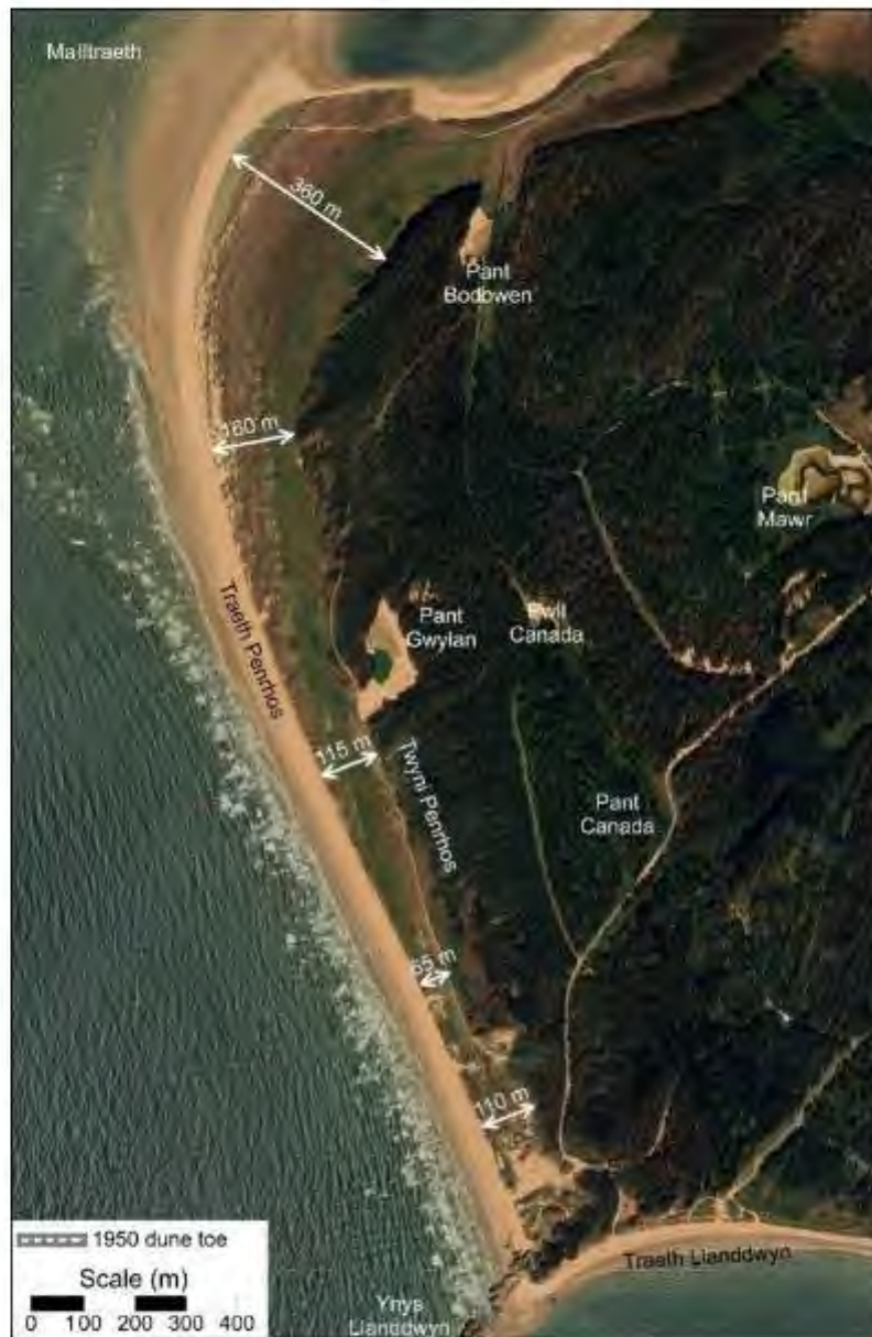
Figure 26. Distance between the dune toe and the edge of forest at present. Base satellite imagery flown 04/07/2023
